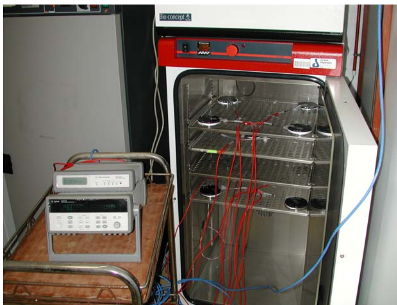
Incubator Characterization (Notice temperature sensors in Petri box)
